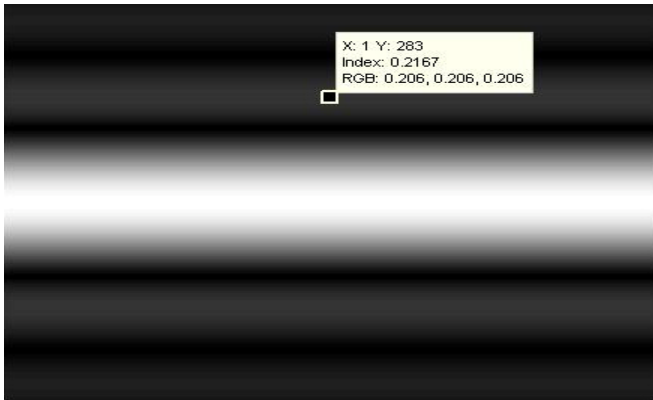
Fig. 3 Simulated Fraunhofer diffraction pattern at the double MC structure
